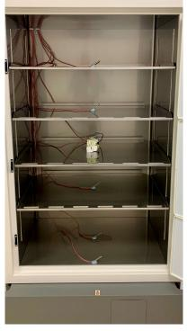
Figure 1. The F740hi with probes positioned at the centre of each shelf. Furthermore, additional probes were positioned at the back of the top compartment (compartment 1) and the front of the bottom compartment (compartment 5). Compartment 3, the middle compartment, had its probes positioned to be exactly at the middle point of the cabinet.
