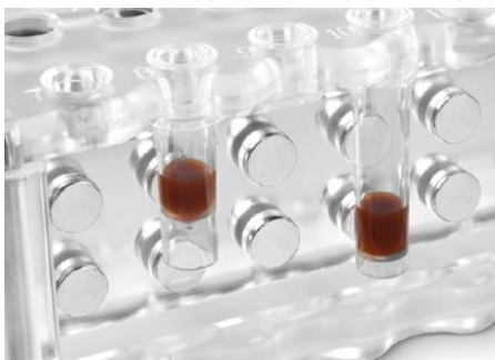
Figure 4. Separation of magnetic beads in tube format
