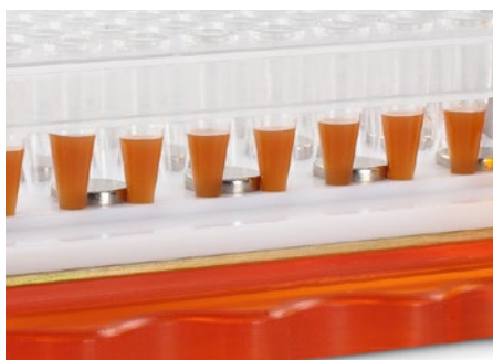
Figure 2. Separation of magnetic beads in microplate format
