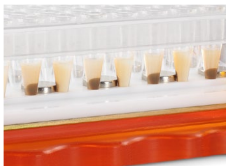
Figure 2. Separation of magnetic beads in microplate format
