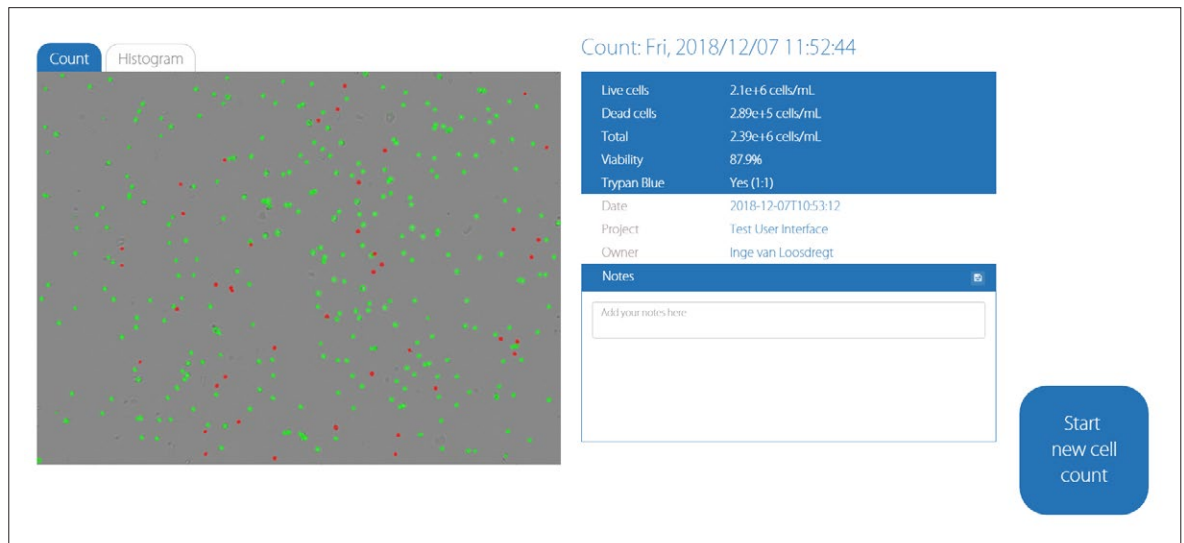
Figure 4. New results page. Click on the “Histogram” tab to view the histogram of the diameter of live and dead cells. The Trypan blue dilution is displayed in the results box.
