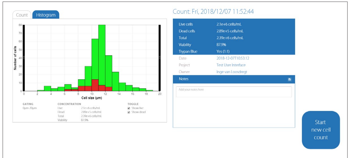
Figure 5. The size histograms of the live and dead cells are displayed in one chart. The histograms can be gated by moving the black bars on the left and right side of the chart.
