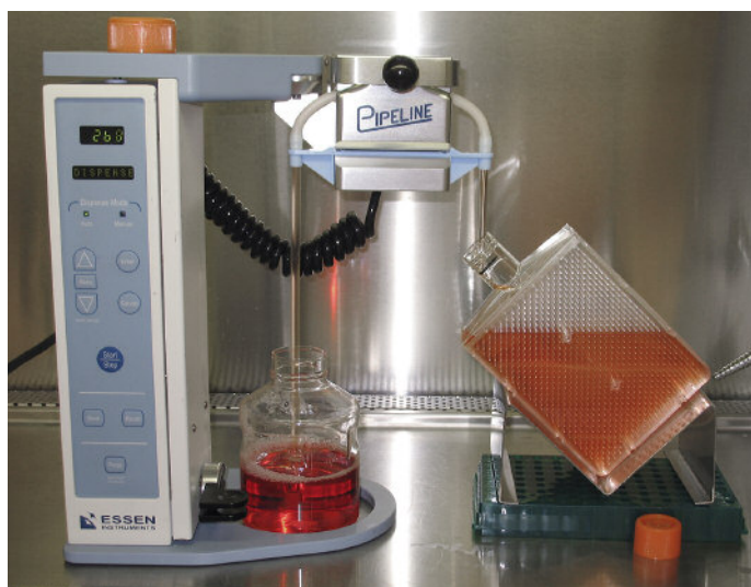
Figure 2. The proper placement and setup of the HYPERFlask vessel and media bottle in the Pipeline™ Dispenser from Essen Instruments, Inc.
