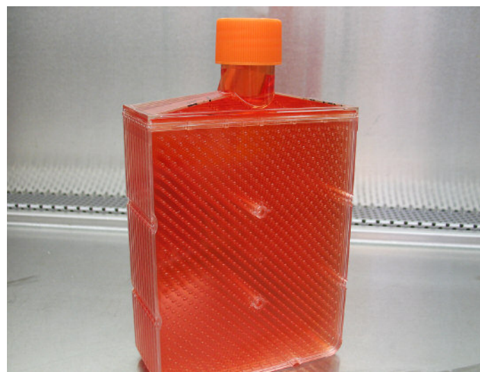
Figure 1. HYPERFlask vessel filled with 565 mL medium.
