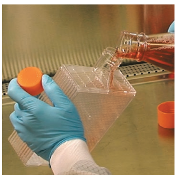
Figure 1. Pour carefully to avoid foaming and bubbles. Notice tilt of flask to achieve low foaming.
