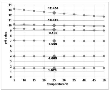
While pH buffer solutions are well known and the pH meters can automatically do temperature compensation (ATC), the temperature behavior of real samples is not known. ATC with samples is normally not possible.
