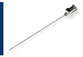
Metal hub (nickel plated brass) needles can be used with TLL syringes and LT or TLL connectors. The needles are 304 stainless steel. Standard needle length is 2" / 51 mm. Metal hub (N) needles are available in convenient six packs. Custom needle lengths and point styles are available.
