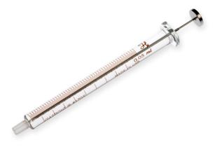
The 1700 series syringes are the Gastight version of the original 700 series syringes. This series of syringes is ideal for dispensing volumes from 1  $\mu$ L up to 500  $\mu$ L. A variety of different terminations and needle options are available in this series.
