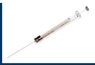
Split/splitless injection consists of a heated chamber with a glass liner into which the sample is injected through the septum. A microsyringe is used to inject the sample through a rubber septum into a flash vaporizer chamber at the head of the column.
