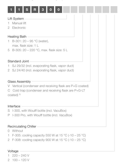
$<sup>^{\</sup>mbox{\tiny 3)}}$  When ordering the glass assembly C, a recirculating chiller is not needed
