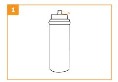
Direct the valve away from you, press it down and turn it clockwise until it is locked.
