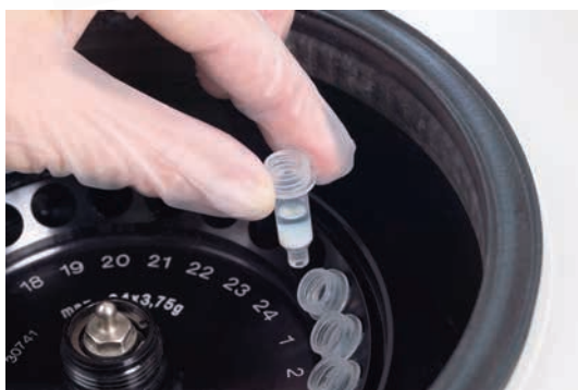
Fig 4. His SpinTrap TALON columns are designed for efficient, small-scale purification up to 1 mg of histidine-tagged proteins.
