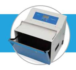
The **Stomacher® 3500** is used where large volume blending is required. The blending of powders with diluents and the microbiological testing of complete recipe dishes are two popular applications.
