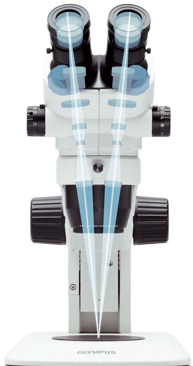
The Greenough optical system has two zoom optical paths inclined at an inward angle. This enables a more compact microscope design while maintaining high performance.
