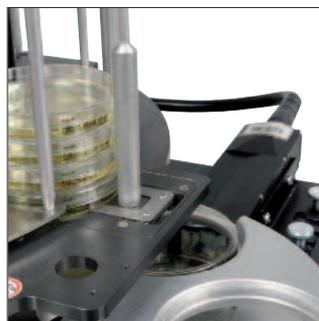
All supported inkjet printers allow side wall imprinting. Alternatively, dishes can be imprinted on the bottom using the LINX 4900 inkjet printer module.
