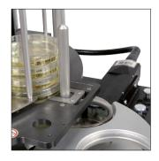
All supported inkjet printers allow side wall imprinting. Alternatively, dishes can be imprinted on the bottom using the LINX 8900 inkjet printer module.
