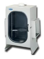
Acoustic Enclosure: Operating a Sonifier® SFX Series in the Soundproof Enclosure can minimize mechanical noise produced by ultrasonic processing. The sturdy cabinet is lined with waterproof, sound-absorbing material, which is impervious to most solutions or laboratory reagents and can be easily cleaned. A fully-transparent door enables viewing of the process while limiting the noise to an acceptable level.
