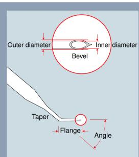
Microcapillaries are complex structures (e.g. TransferTip® (ES)). Producing them is time-consuming, tedious, and costly because it includes multiple steps and instruments.
