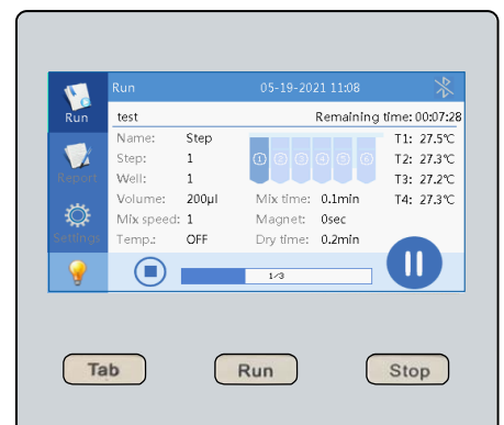
Touch screen control panel
