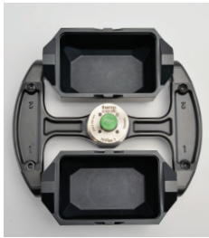
Image 2 - Rotor cross shown with buckets (rotor cross is sold separately, see below for selection)
