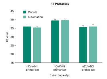
**Fig 7.** Ct values obtained in RT-PCR assay for 200 μL of SeraCare material containing approximately five copies of viral particles/μL processed with Sera-Xtracta Virus/Pathogen kit. Please note that no SARS-CoV-2 specific amplification was detected in the negative control (viral particles containing human RNase P sequence). For clarity, data is not shown. Values averaged from three independent experiments; error bars represent standard deviation
