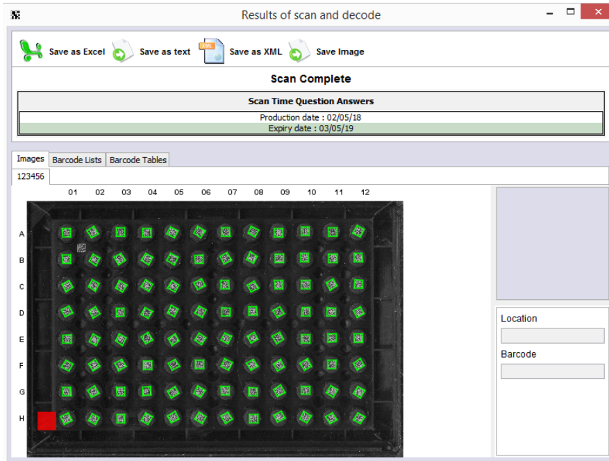
Figure 77: The red error mark shows where DataPaq™ was trying to read the code
