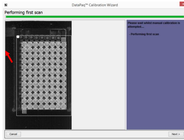
Figure 27: Image of the Rack with a White Overlay
