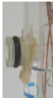
(3) KCl salt crystallization
