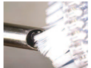
Using Toothbrush to Clean an ISFET pH Sensor
