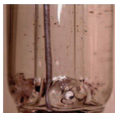
Ceramic Pin Junction Cleared of Sulfide Precipitation by Hach KS410 Solution
