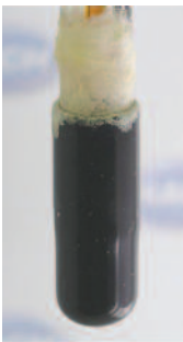
(1) KCl salt crystallization
