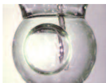
Air in the pH Glass Bulb
