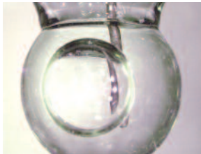
Air in the pH Glass Bulb
