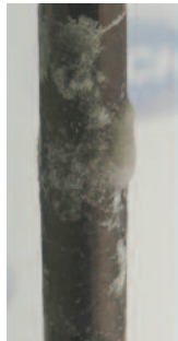
(2) KCl salt crystallization
