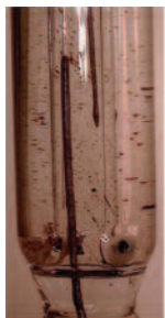
Ceramic Pin Junction Blocked by Sulfide Precipitation
