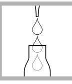
**10.** Pipet into the cooled cuvette: **0.5 mL Reagent B**. Close Reagent B **immediately** after use.
