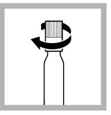
**4. Immediately** screw the DosiCap Zip back on **tight**; **fluting at the top**.
