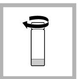
2. Close immediately the reaction tube. Do not invert.
