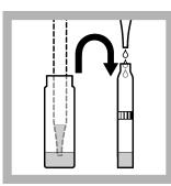
6. Slowly pipet into the Cuvette Test: 0.5 mL of digested sample.
