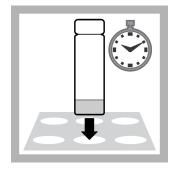
3. Heat immediately. HT 200 S: in the standard program HT for 15 minutes. Thermostat: for 30 minutes at 120 °C (248 °F).
