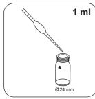
Place 1 ml (25 Tropfen) KS255 (Polyacrylate Reagenz 1) solutionin the test vial.
