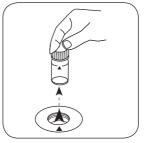
Remove the vial from the sample chamber.
