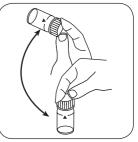
Dissolve tablet(s) by inverting.
