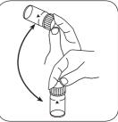
Dissolve tablet(s) by inverting.
