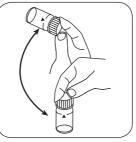
Dissolve tablet(s) by inverting.
