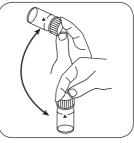
Dissolve tablet(s) by inverting.
