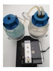
6. Open the lid and place a slide with the chamber side down onto the silicon surface of the slide washing bed. **The holes on the slide should face downwards onto the silicon surface**. Make sure the slide is flush within the chamber. If it is not flush, the system will not operate.
