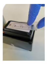
2. Press the slide down simultaneously at both ends to activate the dryer. This will be accompanied by an audible noise of dryer's air pump being activated.
