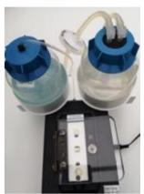
5. Pipette 2ml of silicone defoamer solution into the waste reservoir, then screw on the cap until it is airtight and place in right hand of the white holder.
