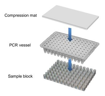
Figure 6. Applying the Compression Mat
