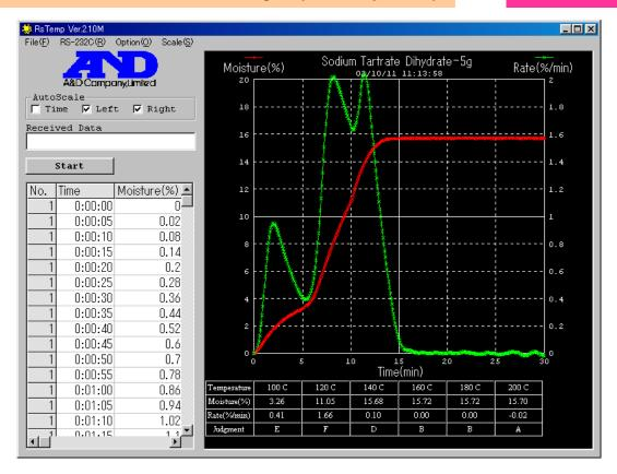
The RsTemp software determines the optimum heating temperature for measuring moisture content with the MS/MX/MF/ML.
