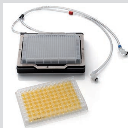
Processing of non-magnetic beads via vacuum filtration module
