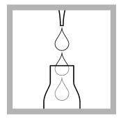
Blank-Cuvette: Carefully pipet 2.0 mL of deionized water (blank).
