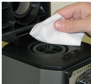
FIGURE 4.21 CLEANING INTERIOR SURFACES
