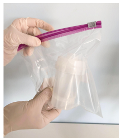
FIGURE 4.18 ASSEMBLY IS BAGGED AND READY FOR TRANSPORT TO THE LABORATORY
