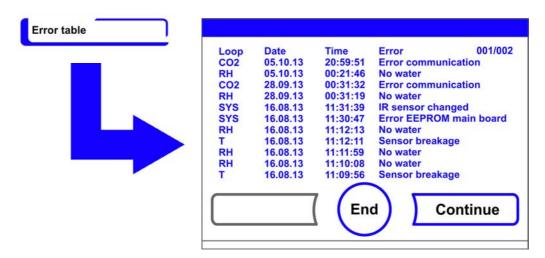
Figure 6-34. Displaying the Error Table
