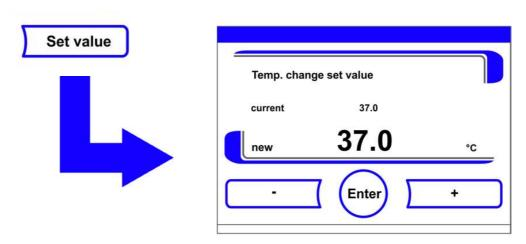
Figure 6-8. Setting the Temperature Set Value
