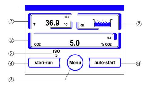
Figure 6-3. iCan™ Touchscreen without O<sub>2</sub>/N<sub>2 gas supply</sub>
