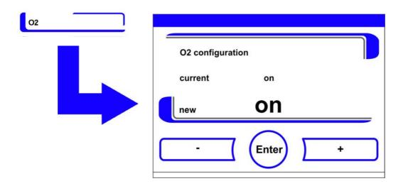
**Figure 6-42.** Switching the O<sub>2</sub> Control on and off
