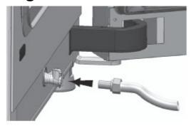
Figure 3-13. Fill and Drain Valve Incubator
