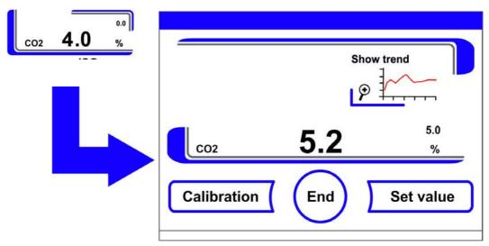
Figure 6-48. Invoking the CO<sub>2</sub> Concentration Graph Display
