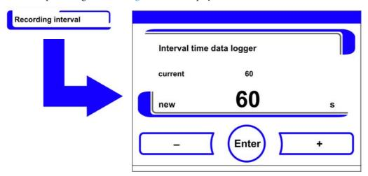
Figure 6-33. Logging Cycle Setting
