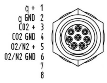
Figure 4-15. Pin-out of the 4-20 mA Interface
