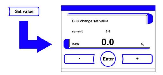
**Figure 6-10.** Setting the CO<sub>2</sub> Set Value
