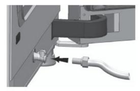
Figure 5-2. Fill and Drain Valve Incubator
