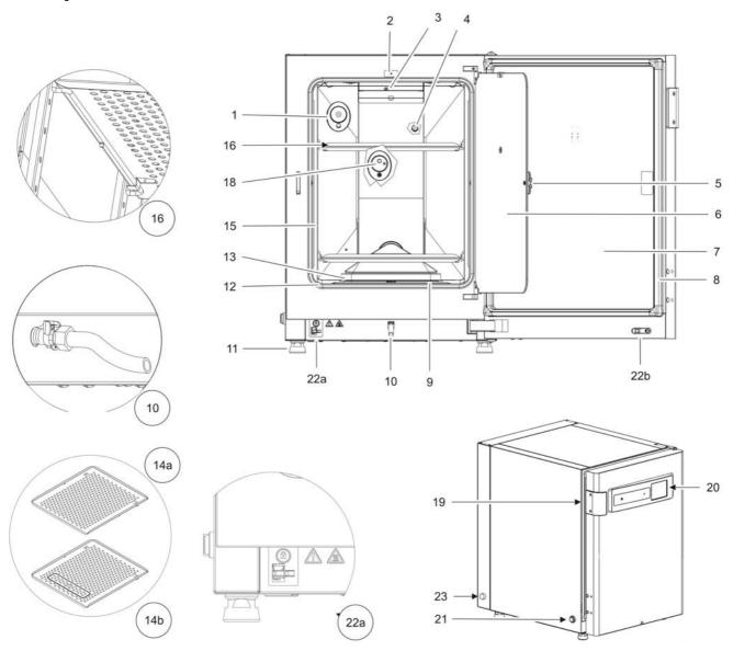
Figure 3-1. Steri-Cycle i160 / i250 CR Front View
