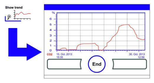
Figure 6-49. Invoking the CO<sub>2</sub> Concentration Graph Display
