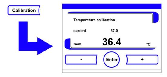
Figure 9-3. Temperature Calibration Procedure
