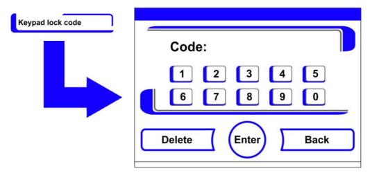
Figure 6-19. Changing the Keypad Lock Code
