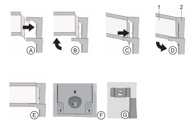
Figure 4-3. Assembling the Air Duct
