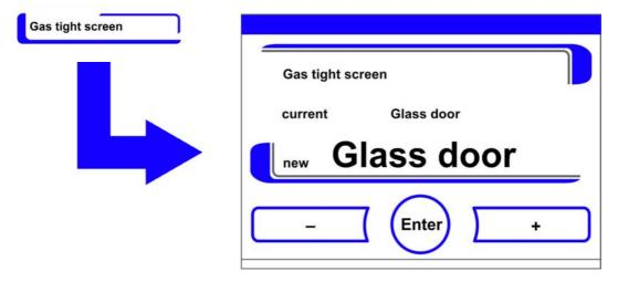
Figure 6-39. Setting the Gas Tight Screen
