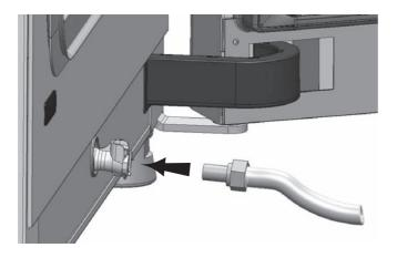
Figure 7-1. Fill and Drain Valve of Water Reservoir
