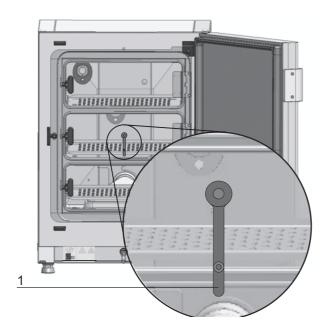
Figure 9-4. Gas-Tight Screen Measurement Opening
