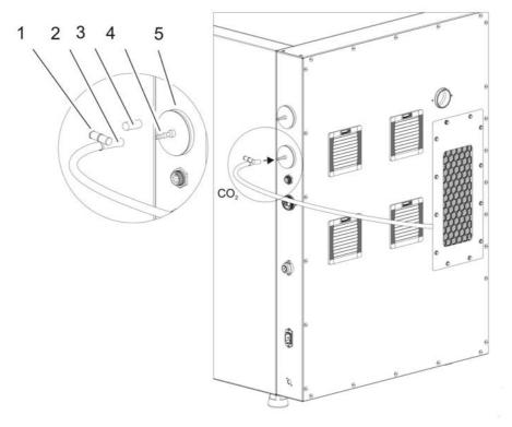
Figure 4-11. Installing Gas Pressure Hoses
