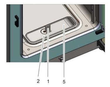
Figure 5-4. "MAX" Fill Level Indicator
