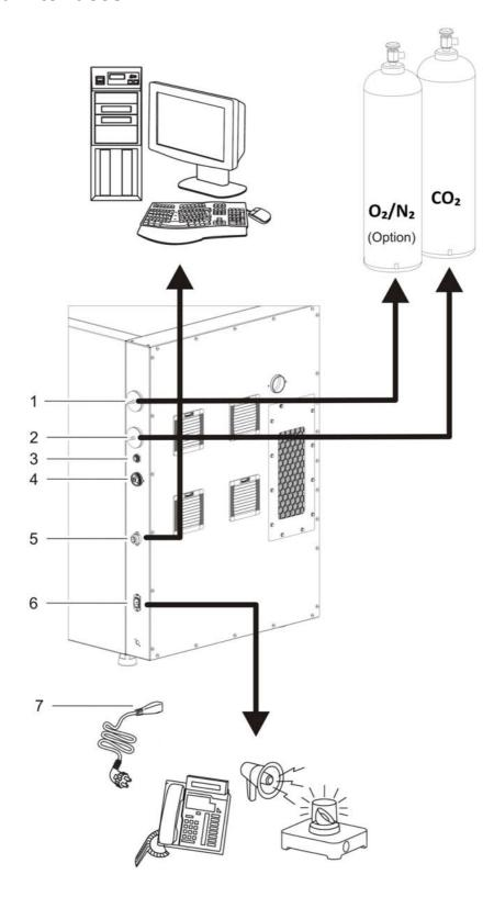
Figure 3-8. Interfaces (Right Side of Control Box)
