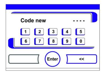
Figure 6-20. Changing the Keypad Lock Code
