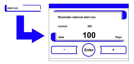
Figure 6-30. Setting the Reminder Interval for Steri-run
