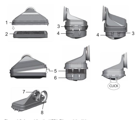
Figure 4-5. Assembling the HEPA-Filter and the Airbox
