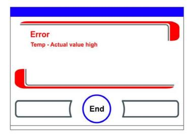
Figure 6-52. Failure Message Overtemperature
