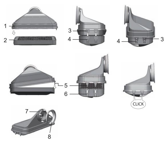
Figure 9-7. Installing the HEPA-Filter
