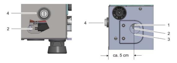
Figure 8-9. Door Lock Latch and Emergency Release on Underside of Incubator
