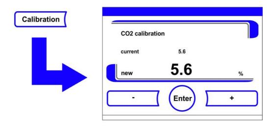
Figure 9-5. CO<sub>2</sub> Calibration Procedure
