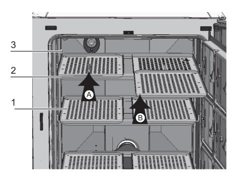
Figure 4-10. Installation of Split Inserts
