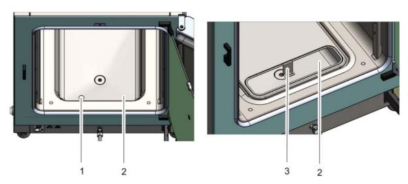
Figure 3-7. Sensors for Water Level
