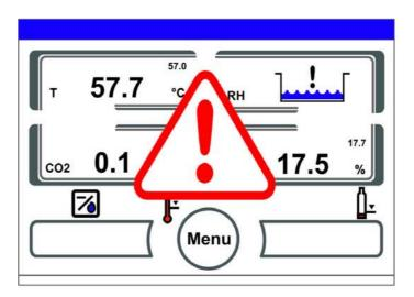
Figure 6-51. Failure Message Overtemperature
