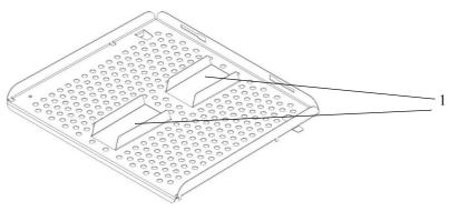
Figure: Perforated Shelf with Separated Guiding Rails for the Lower Position This guiding rails cannot be removed.
