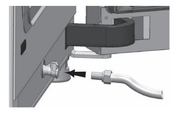
Figure 3-12. Fill and Drain Valve of Water Reservoir
