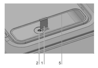
Figure 4-1. "MAX" Fill Level Indicator
