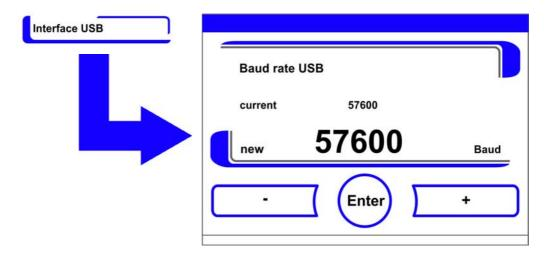
Figure 6-27. USB Interface Baud Rate Setting
