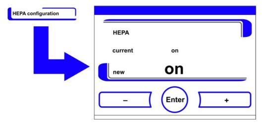
Figure 6-44. Activating / De-Activating the HEPA-Filter
