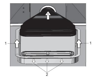
Figure 4-7. Installing the Airbox
