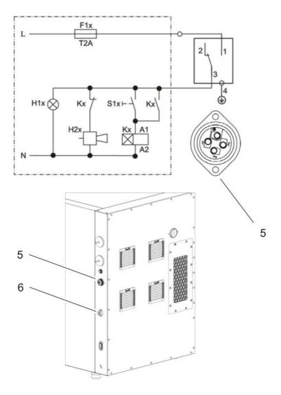
Figure 4-14. Connection Example Alarm Contact
