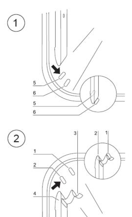
Figure 4-8. Support Rail Installation/Removal
