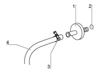
Figure 9-8. Gas Inlet Filter Installation
