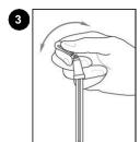
3. Activate Device. Bend bulb, breaking Snap-Valve
