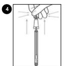
Lift bulb up (about 1 – 2 inches) and squeeze bulb to release liquid into bottom of tube. Replace bulb on 10 tube. Liquid should now be in bottom of tube.
