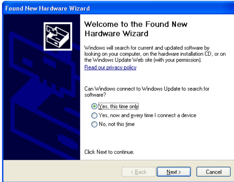
Figure 44 - Found New Hardware for Serial Converter
