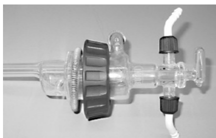
Fig. 25: Glass oven with sublimation accessory
