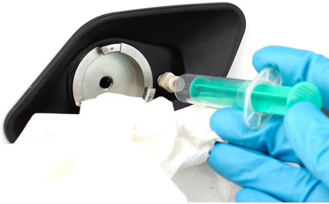
Fig. 30: Rinsing the measuring cell from the outlet
