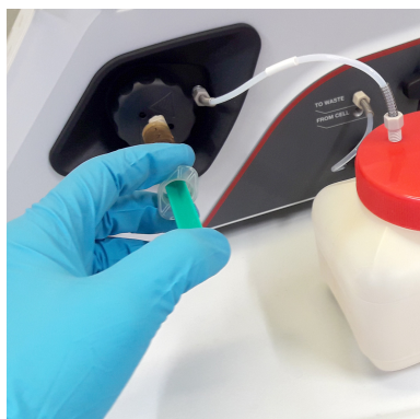
Fig. 18: Filling sideways with a 5 mL syringe
