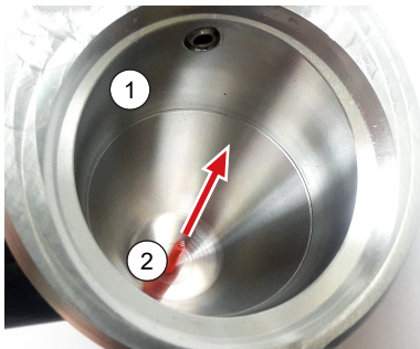
Fig. 9: Removing the bend protection of the funnel hose
