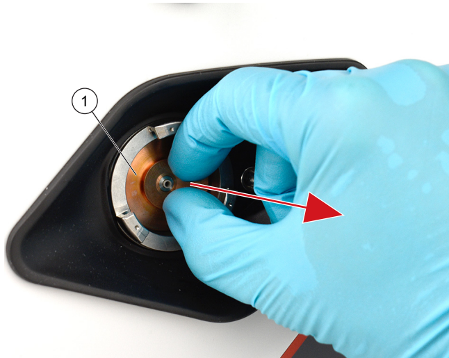
Fig. 26: Taking out the measuring rotor
