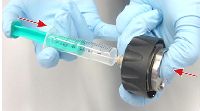
Fig. 22: Leak test measuring cell lock
