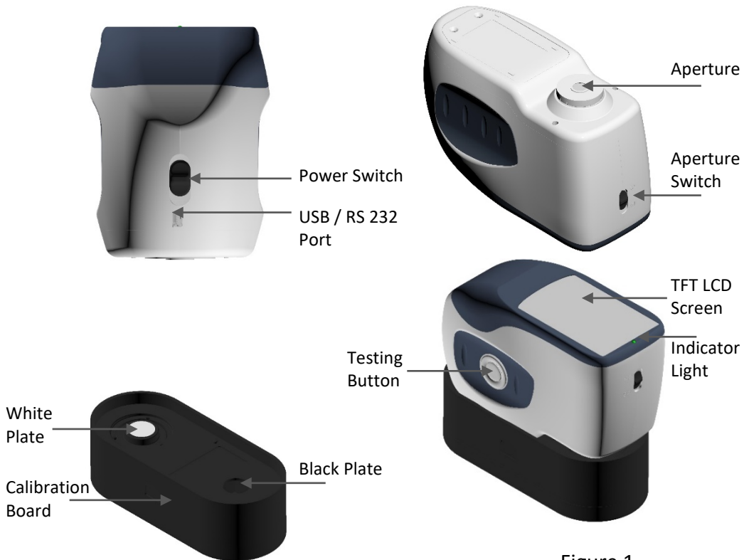
Figure 1 Instrument Structure Diagram
