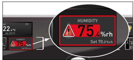
Fig. 22 Humidity monitoring triggered
