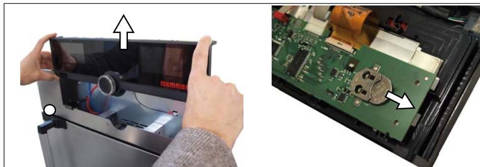
Fig. 34 Removing the lithium battery
