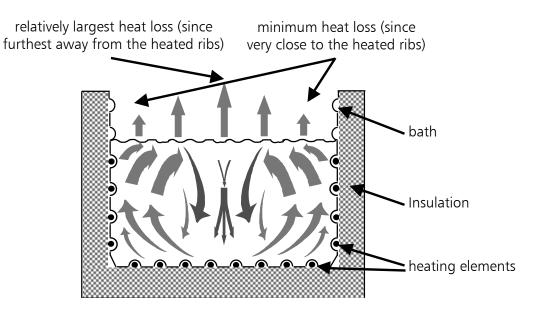
The heating positioned on three sides around the tank ensures a natural water circulation of the liquid inside, thus securing an optimal uniform temperature distribution.
