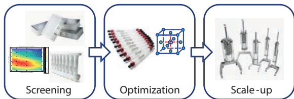
Fig 4. The recommended workflow is described in the figure. It starts with screening of conditions in high throughput formats, followed by optimization, preferably by applying Design of Experiments (DoE), in small columns and finally scale-up to large columns.
