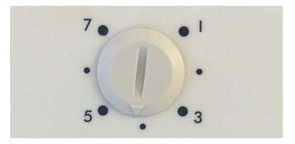
Such dials are simply numbered with the numbers not corresponding to any temperature. Having temperature monitored dial controlled unit it has been observed that the internal temperatures may be as cold as -38°C. This case study aimed to highlight the energy which could be easily saved by using a laboratory freezer at -20°C.
