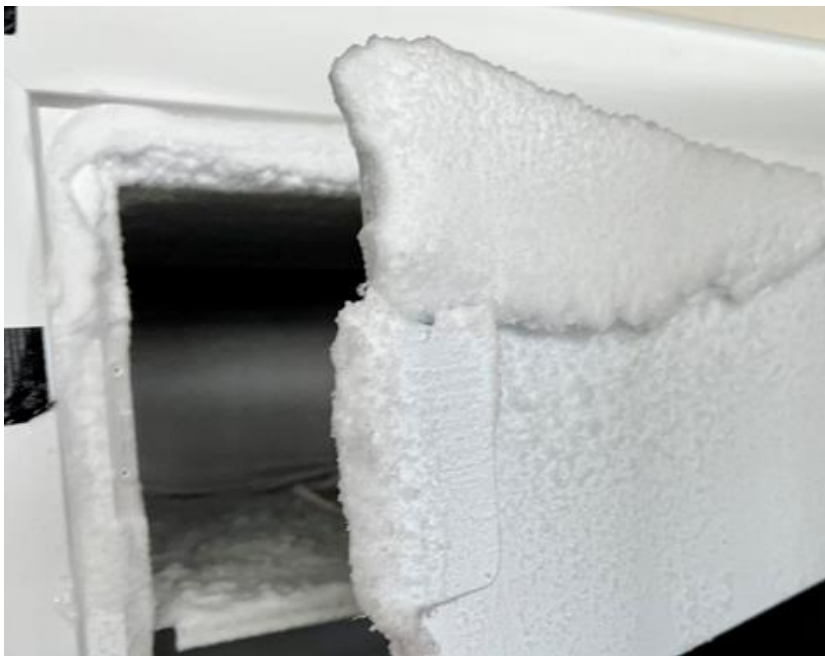
Figure 12. Icing build up progressed throughout the testing steps when the door seal was obstructed and was localized to the inner door and door frame of compartments 1 & 2.
