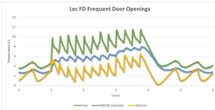
Figure 8. Frequent door openings of the Lec fridge.
