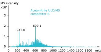
The mass spectra of these four different acetonitrile grades clearly shows the variation in the intensity of the reserpine signal ([M+H]+=609), as well as the extent of the background signals. The differences in the intensity of the reserpine signal are caused by ion suppression. This effect occurs due to interfering trace contaminants that can be present in acetonitrile, which can be avoided using the correct high grade solvent for this purpose.
